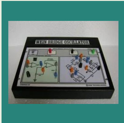
Transistor Wien Bridge Oscillator
